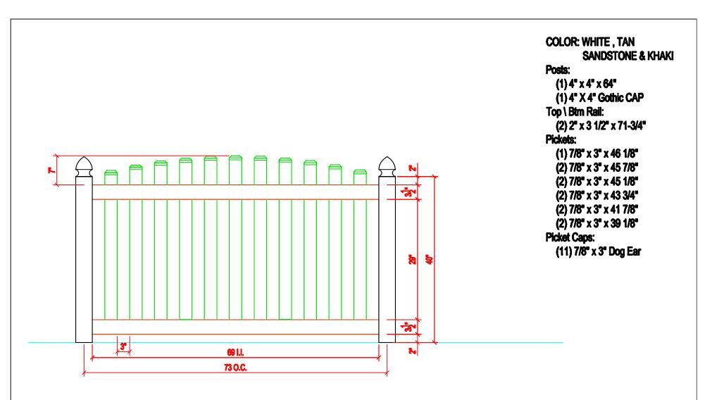
Picket spacing will vary 1/2"+/- based on panel widths. Installation will be full manufacture panels with partial panels on end to complete runs.
