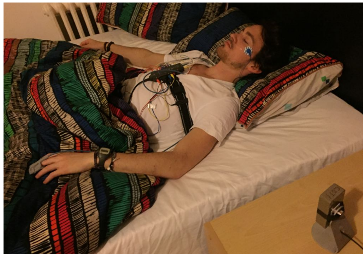
Figure 5. Set up of participants during the study. Polysomnography equipment is strapped to the participant. The Circadia Contactless Sleep Monitor (bottom left) is collecting data wirelessly from the nightstand.
