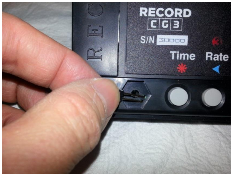
Figure 4: Activating the Config Switch, using the rate-set pin. Contact must be made with the two copper-plated holes on the circuit-board inside the taximeter case, in order to short the holes together..
