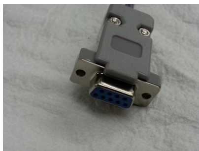
Figure 2: D9 Serial Connector. Used for RS-232 communication. You will need a male 9-pin Connector if you are using a Black Cat adapter for sensing motion, or a female connector if you are communicating with most Dispatch Terminals (MDT). IMPORTANT: See section 2.2
