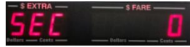
Figure 5: The Security Code Prompt, which locks against proceeding to programming mode when an optional security code has been previously set.
