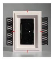
11. For knockout and wiring, press on the soft pre-punched 1/2" and 3/4" knockouts on the junction box. Re-check the electrical box to ensure it is centered with the gypsum platform after wiring.
