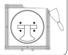
6 Sand surface smooth. Apply one coat of primer and wait for it to dry. Apply two coats of paint (it is recommended that you paint inside of the opening).
