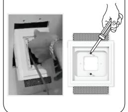
**4** \*ATTENTION: make sure to install the platform upward to position the screw openings on the mount at the top and bottom. DO NOT INSTALL SIDEWAYS.
