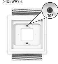
**5** Cover the inside of the platform with paper or tape to protect the center opening. Apply the fiberglass tape on all four joints around the platform. Patch with drywall compound.
