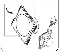
4 Level the drywall with the lower line of the joint on the front of the gypsum platform. Secure SeeLess platform using flat headed drywall screws.
