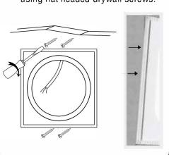
**5** Cover the inside of the platform with paper or tape to protect the center opening. Apply the fiberglass tape on all four joints around the platform. Patch with drywall compound.
