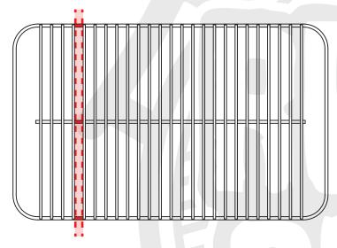
2 ALIGN THE HINGE PLATES TO THE COOKING GRATE WITH THE WAVY PLATES ON TOP & FLAT PLATES ON THE BOTTOM.
