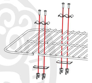
FASTEN THE HINGE PLATES TO THE GRATE USING THE BOLTS & WING NUTS PROVIDED.
