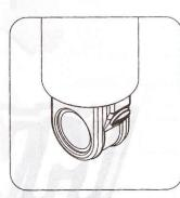
Rebound adjustment knob + direction rotation, increase damper (slow) - direction rotation, decrease damper (fast)
