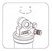
1 Main air chamber Supply air pressure according to pressure meter
