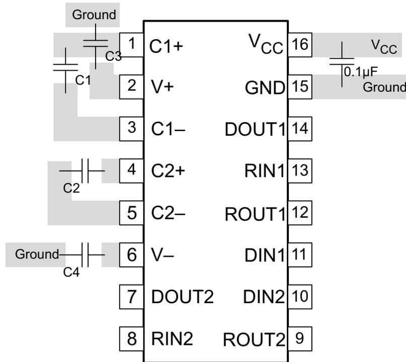
**Figure 8. Layout Diagram**
