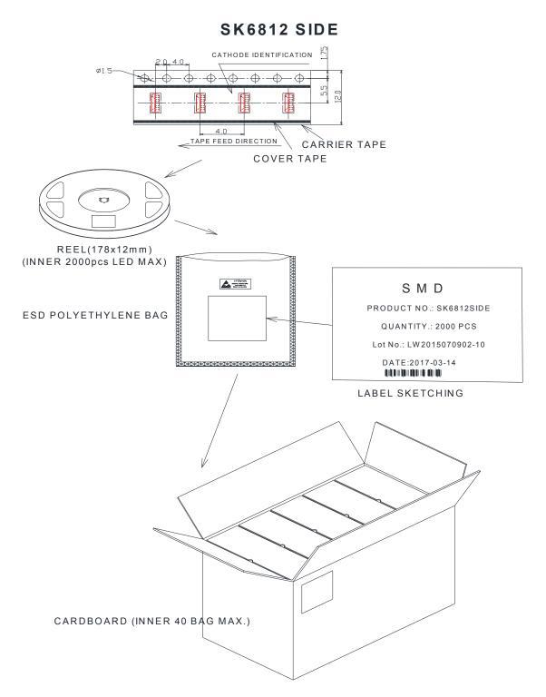
The reel pack is applied in SMD LED. The LEDs are packed in cardboard boxes after packaging in normal or antielectrostatic bags. cardboard boxes will be used to protect the LEDs from mechanical shocks during transportation. The boxes are not water resistant and therefore must be kept away from water and moisture.
