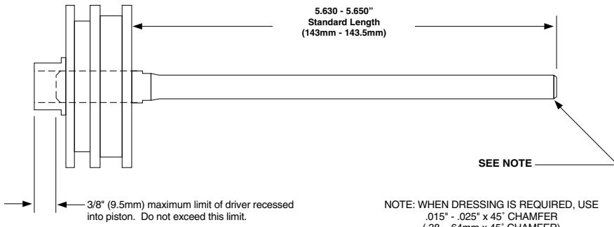
**NOTE:** Driver wear of approximately 1/8" (3mm) can be tolerated in most applications. However, in difficult driving applications, driver wear or approximately 1/16" (1.5mm) may cause a slight reduction in the apparent driving power.
