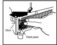
1. **Open the canister:** pull down down latch and swing door open. Swing canister cover open.
