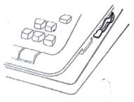
The machine should be replaced in the case before carrying it any distance. Set the machine on the prongs at the rear of the baseboard, then press into the spring clips at the sides. Insert the case cover into the rear hinges of the baseboard, close and lock.
