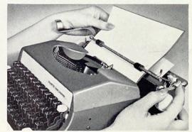
If the paper has not been fed through perfectly straight it can be adjusted by pushing back the paper release lever to its full extent. This frees the paper so that the edges may be levelled after which the paper release lever should be returned.
