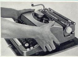
Although the machine may be used on the baseboard it can be removed if desired by grasping as shown and depressing the stud on each side of the machine with the forefingers and lifting clear. The machine has its own rubber feet which will not scratch or harm the surface of the desk or table.
