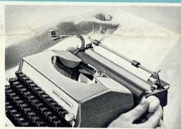
Lift bail bar to its full extent by means of the bail bar lever. Place the paper on paper shelf close up to paper locating guide. Rotate platen knob away from you and the paper will emerge from the front of the platen roller. Pull bail bar forward, over the paper and adjust the auxiliary feed rollers.
