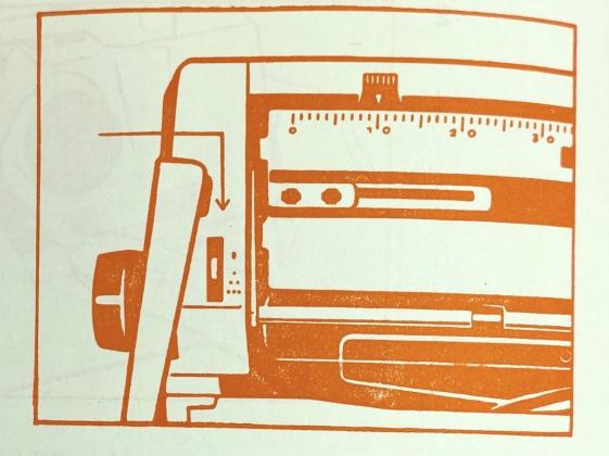
Line adjusting device and platen release The lever (16) (Fig. 3) has a double function; in the rear position (1) it release the platen. The further symbols mean:
