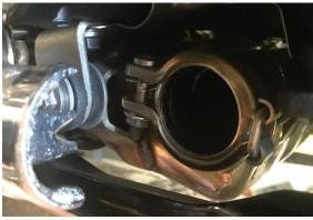
7. Tighten clamps on catalytic converter to 8 Nm. (70 in-lbs) NOTE INCH-POUNDS
