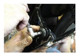
3. Use 5mm allen to loosen heat shield.
