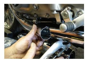
5. Use 10mm deep socket or 10mm wrench and loosen the mid-pipe catalytic converter clamp under the motorcycle.
