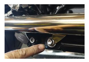
6. Use 10mm deep socket or 10mm wrench and tighten the catalytic converter clamp under the motorcycle.
