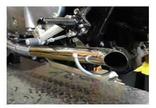
Before starting motorcycle, check for proper clearance between new exhaust system and rear suspension (i.e. tire, swing arm, brakes, rear shock, and etc.) If any problem is found, please carefully follow through the installation steps again. If problem still persists, please call **British**Customs Customer Support at (877) 999-2748.
