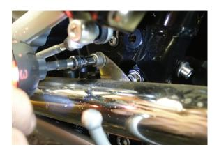
On right side, use factory mounting bolt to secure Performance Tip. Use 12mm socket to tighten and torque to 19 Nm (14.0 ft-lb)
