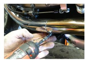
Left side, use 6mm allen and tighten rear mounting bolt. Torque to 14 Nm (10.0 ft-lb)
