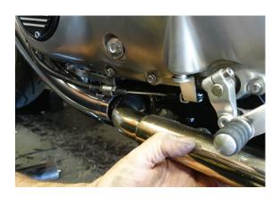
2. Lift Performance Tip into place and install supplied 8mm x 16mm socket head bolt into factory location.
