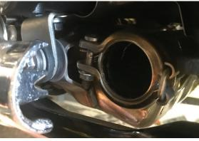
Use 12mm socket to remove midpipe mounting bolt under ride pegs. (Save bolt on right side.)
