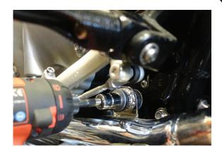
7. Pull the mid-pipe outward, away from the motorcycle, until it is free from the catalytic converter.
