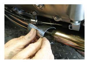
4. Use 5mm allen and tighten heat shield clamp to 9 Nm. (80 in-lbs) NOTE INCH-POUNDS
