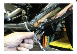
2. Use 6mm allen and 12mm wrench to remove rear muffler mounting hardware and remove muffler.
