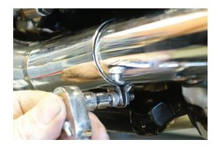
Remove heat shield by pulling the rear and sliding toward the back of the motorcycle.
