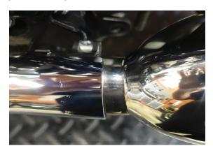
8. Tighten heat shield 5mm allen clamp firmly.
