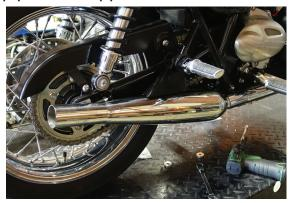
5. Position mounting bracket of Sleeper to rear of passanger foot peg mount.
