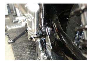
7. Tighten 5mm allen clamp securing Sleeper to headpipe to 10 Nm. (7.38 ft-lb)
