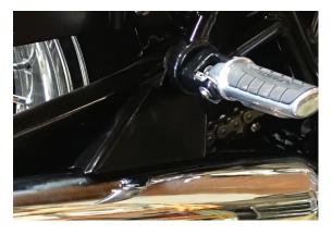
Install supplied spacer over passanger peg bolt, the 12mm nut, then tighten. Torque nut to 19 Nm (14.0 ft-lb)
