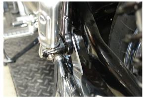
Tighten clamp securing Predator Pro to headpipe to 10 Nm (7.38 ft-lb)
