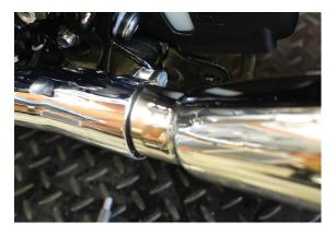
6. Tighten heat shield 5mm allen clamp firmly.
