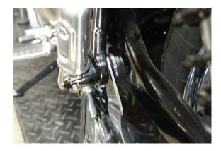
5. Tighten clamp securing GP Slip-on to headpipe to **10 Nm (7.38 ft-lb)**
