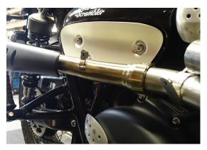
Position upper silencer onto upper head pipe (left hand), insert the rear 12mm mounting bolt and tighten, but do not torque at this stage.
