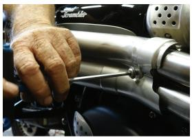
On back side of headers, tighten and torque tabbed clamp to 10 Nm. (7.38 ft-lb)
