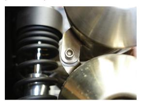
Position the silencer clamps, securing silencers to the head pipes and torque to 10 Nm. (7.38 ft-lb)
