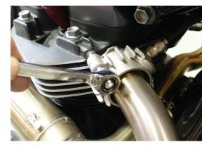
11. Tighten and torque left hand head pipe clamp (behind radiator) to **10 Nm. (7.38 ft-lb)**
