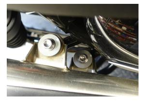
15. Position only the inner heat shield cover of the center heat shield to the silencers, fit the shouldered washers, insert only the rear screw, and tighten.
