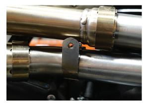
14. Tighten the silencers rear mount bolts with 12mm socket and torque to **19 Nm. (14 ft-lb)**
