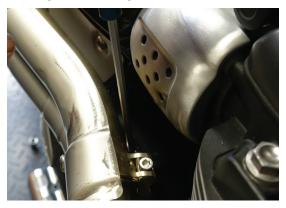
19. Remove the two screws and shoulder washers from center heat shield.
