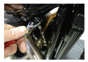
Fit the 5mm screw securing the rear of the exhaust silencers together and tighten to 10 Nm. (7.38 ft-lb)
