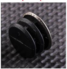
The idea of the whole procedure is to block the AIS ports on the cylinder heads with the provided block off plugs, block the AIS carburettors vacuum ports with the vacuum cabs, and plug the airbox port of the AIS system plastic cap included in the kit.
