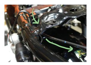
2. Locate rear seat latch assembly to the rear sub-frame position.
