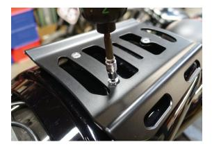
3. Use 6mm allen to remove rear rack bracket and seat cowling.
