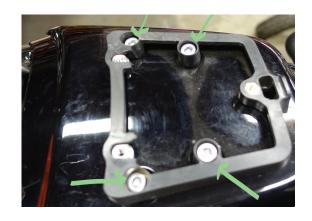
Use T30 Torx to loosen the four fender mounting screws. Support rear fender, continue removing screws until fender drops free. Fender screws and leaves do not need to be removed.
