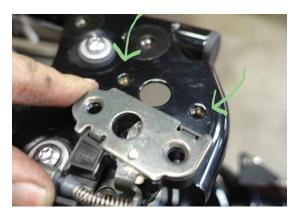
Use T30 Torx and factory hardware to secure seat latch assembly to sub-frame. Torque to 6 Nm (53 in-lbs.) \*INCH-LBS
