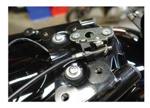
4. Lift and secure fender with factory T30 Torx screws. Torque to 10 Nm (88 in-lbs.) \*INCH-LBS
