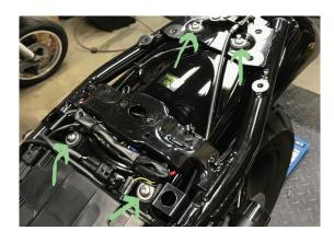
5. Install Slammer Seat and push down on the rear to engage seat latch.
