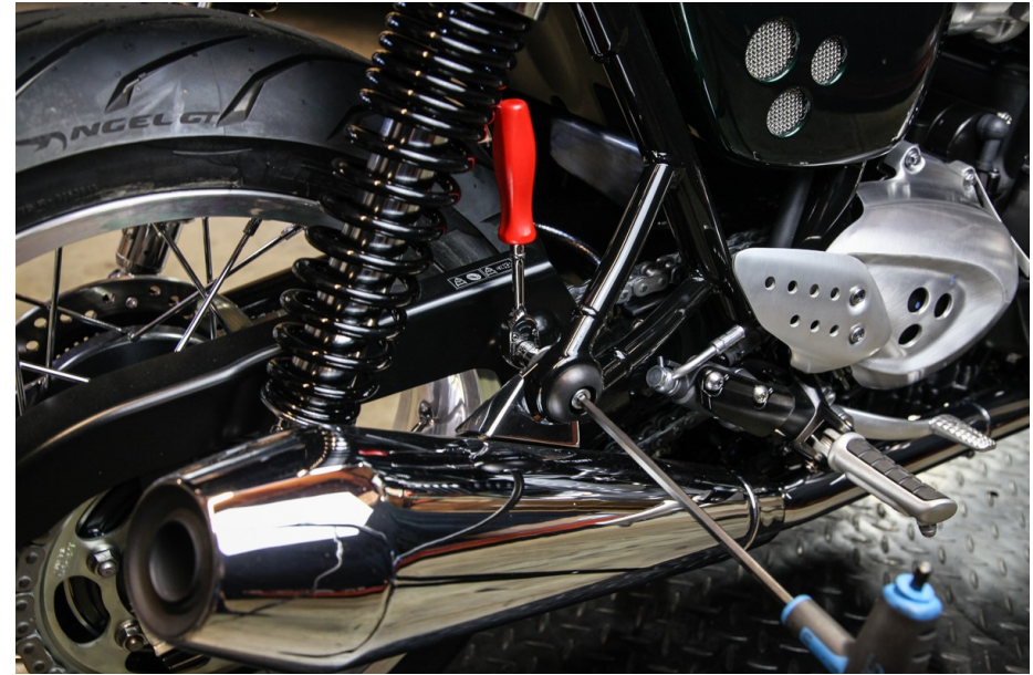
STEP 3: Use a 6mm Allen wrench and a 10mm socket wrench to remove the stock rubber passenger peg block off.
