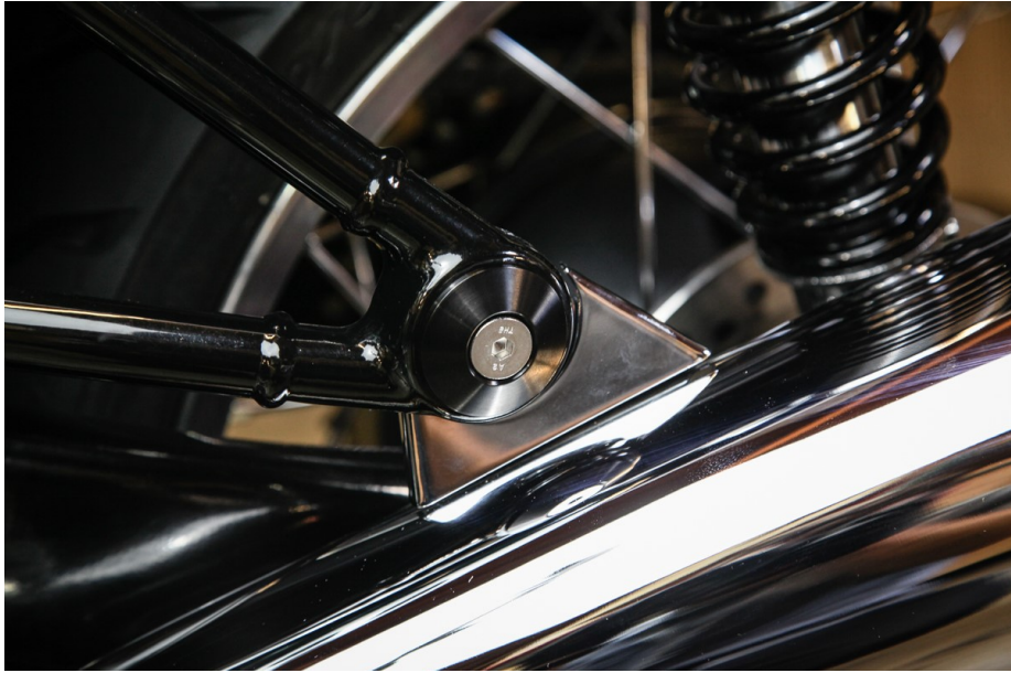
This is what the Mule Passenger Peg Block-Off looks like after successful installation.
