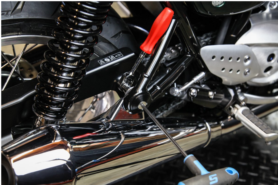
STEP 4: Use a 5mm Allen wrench and a 10mm socket wrench to install the Mule Passenger Peg Block Offs. Reuse the stock nut to install.
