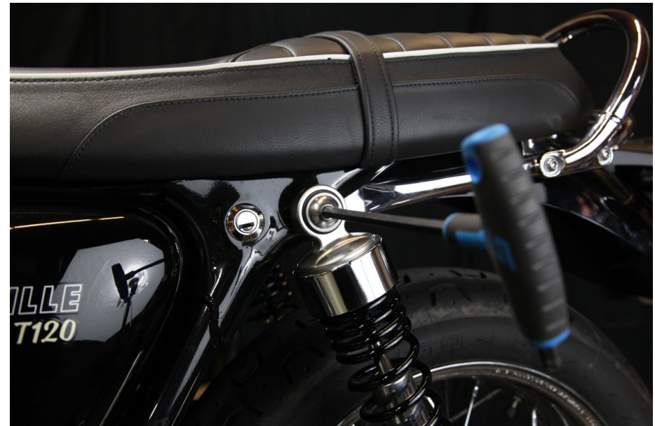
STEP 1: Remove only one shock bolt at a time, otherwise you may damage your motorcycle or injure yourself by causing the motorcycle to fall. Use an 8mm Allen wrench to remove the stock left upper shock bolt and washer.
