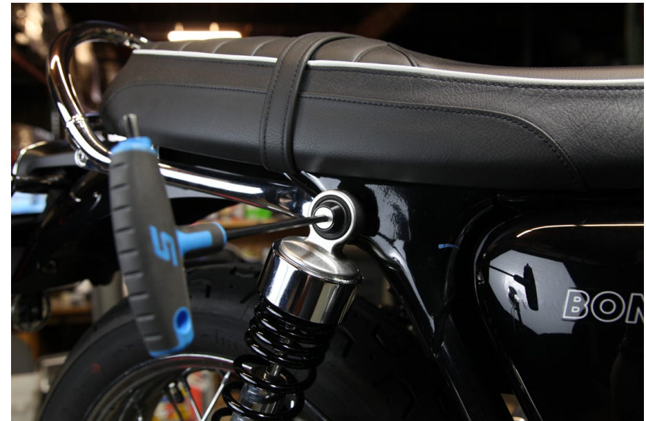
STEP 7: Use a 5mm Allen wrench to install the shock hardware dress up bolt and spacer. Torque to 28 Nm.
