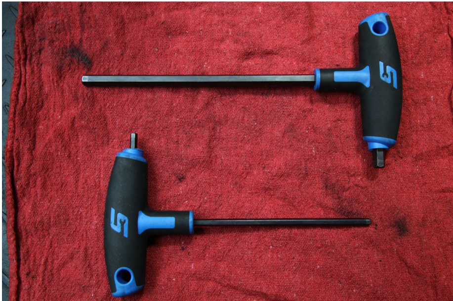
PREP: For this installation, you will need a 5mm and 8mm Allen wrench.
