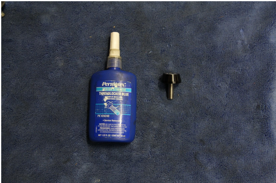
STEP 2: Insert the supplied bolt into the spacer, and apply blue Loctite or medium threadlocker.
