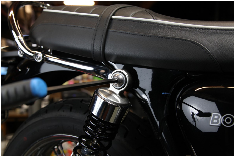
STEP 6: Use an 8mm Allen wrench to remove the stock right upper shock bolt and washer.
