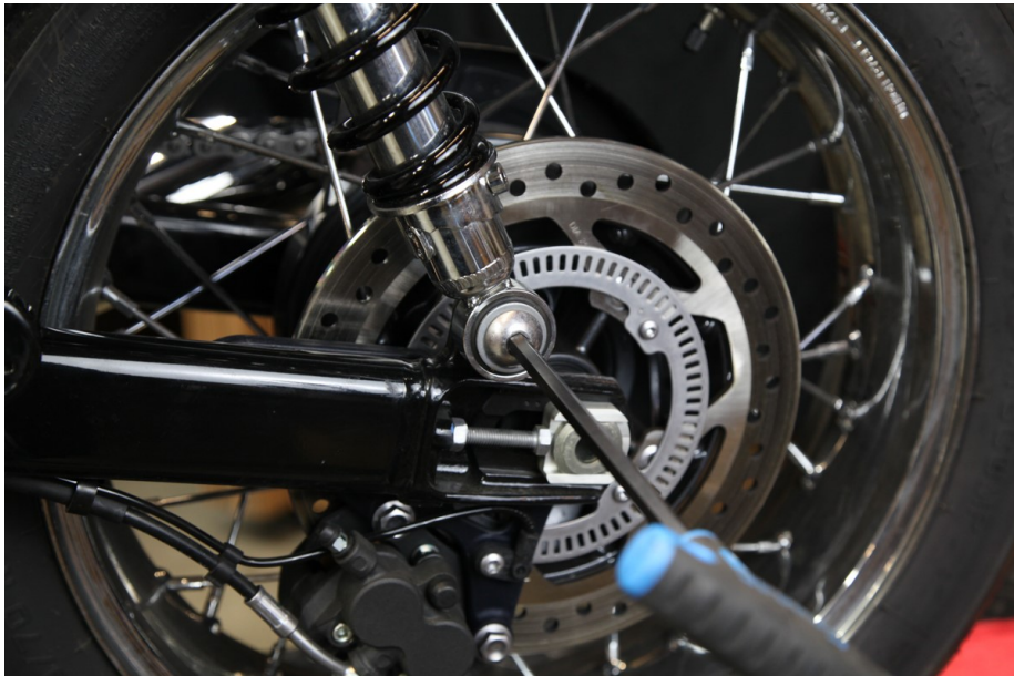
STEP 4: Use an 8mm Allen wrench to remove the stock left lower shock bolt and washer.
