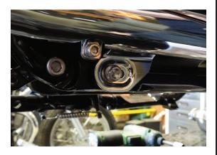
13. Tighten clamps securing right header pipe to X-pipe to 10 Nm. (7.38 ft-lb)
