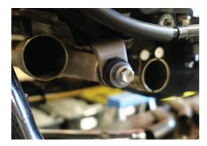
3. Position left cradle into place, ensuring radiator lower mounting hole lines up with mounting post on the inside of the cradle.
