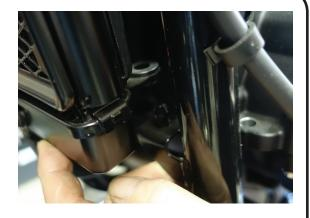
4. Fit the cradle assembly two rear mounting bolts and nut plate, do not fully tighten at this stage.
