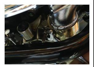
14. Locate the left exhaust header pipe to the cylinder head. Fit the two 12mm nuts and the finned clamps securing the left hand header pipe to the cylinder head, do not fully tighten at this stage.
