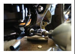
5. Fit the 8mm allen bolt and 14mm nut securing the cradle to the headstock. Torque to **40 Nm. (30 ft-lb)**
