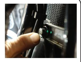
2. Remove the left hand side crankcase front mounting hardware using T-55 Torx driver and 17mm wrench on the nut.
