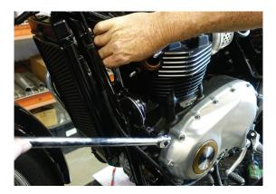
8. Fit 10mm bolt to upper radiator bracket and torque to 8 Nm. (5.9 ft-lb)
