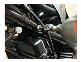
Remove the two 8mm allen bolts at the rear of the left hand cradle and collect the nut plate.
