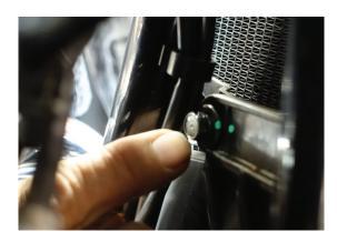
9. Locate the right exhaust header pipe to the cylinder head. Fit the two 12mm nuts and the finned clamps securing the right hand header pipe to the cylinder head, do not fully tighten at this stage.
