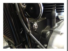
3. Remove 8mm allen and 14mm nut securing the left hand cradle to headstock.
