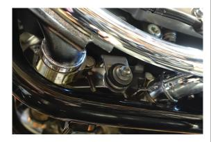
18. Route the oxygen sensor harness and connect to the main harness as noted for removal.
