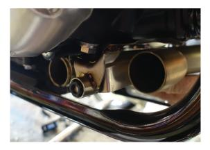
2. Fit 12mm bolt on the side of the x-pipe and torque to **15 Nm. (11 ft-lb)**
