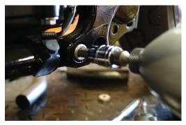
5. Support the left hand cradle assembly and gently lower the cradle assembly, taking care not to pull on the side stand sensor wire at the rear of the cradle.
