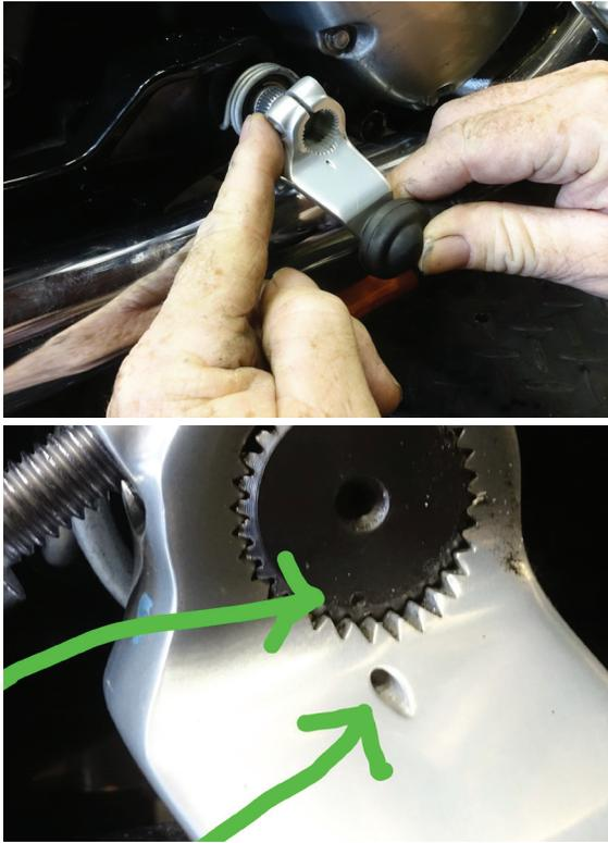
12. Use 5mm allen and torque Rear Brake Clevis bolt to **5 Nm (16.0 ft-lb)**
