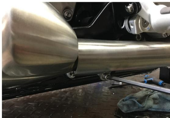
4. On Streetmaster Models, Use 5mm allen and remove the Rear Brake Lever Clevis Bolt and slide clevis off shaft. Gently move clevis and linkage out of the way.
