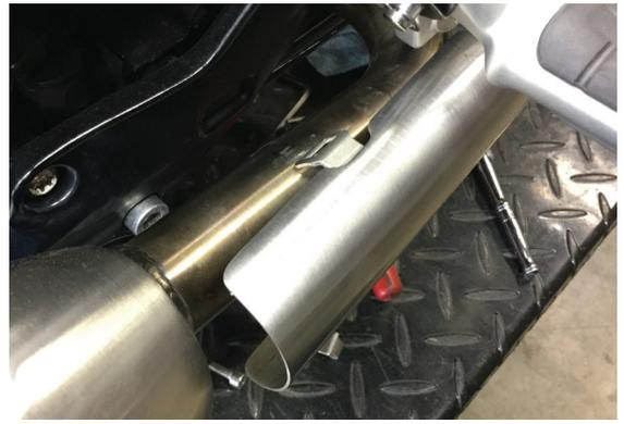
7. Pull Silencer outward, away from the motorcycle, until it is free from the catalytic converter and rear mount bracket. Swing silencer end down and remove from motorcycle.
