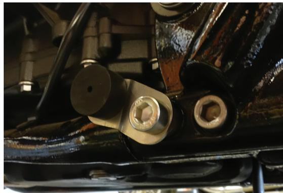
4. Cycle the kickstand to get the bracket into proper position, then tighten and torque to **40 Nm. (30 ft-lb)**
