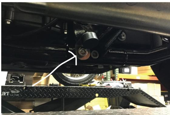
3. Place kickstand stopper bracket into position and secure with supplied 8mm allen.
