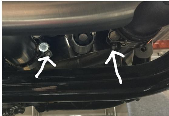
3. Use 5mm allen to remove the heat shield clamp bolt. (On the left hand side, remove the heat shield mid-section.)
