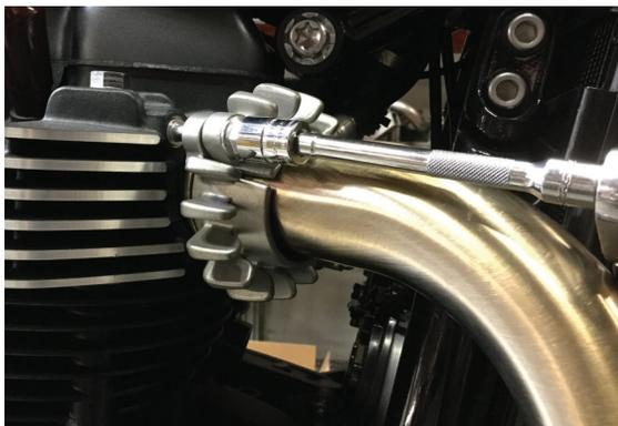
8. Tighten clamps on catalytic converter to **8 Nm. (70 in-lbs)**
