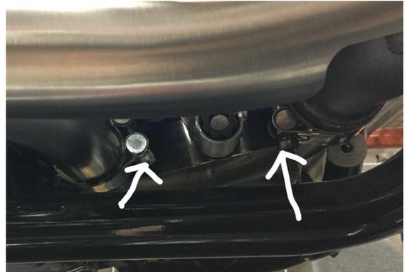
9. Install heat shield to tailpipe. Tighten clamp firmly with 5mm allen and torque to **9 Nm. (80 in-lbs)** **NOTE INCH-POUNDS**
