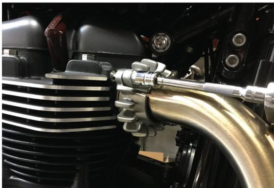
2. Loosen the Four (4) clamps on the catalytic converter with 10mm wrench.
