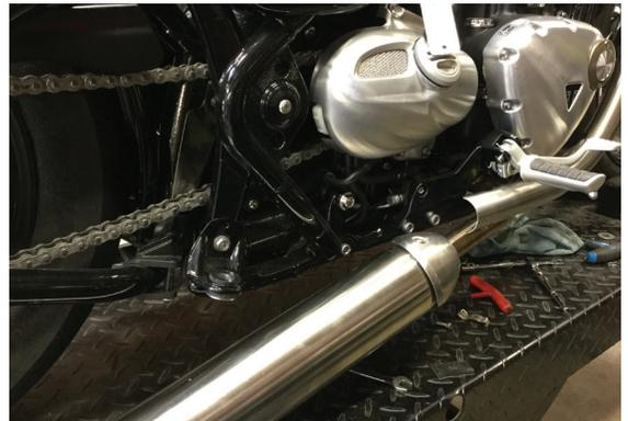
8. Use 12mm socket to remove the rear muffer mounting bracket.
