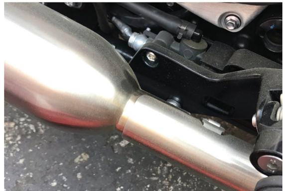
10. Go to rear mount and tighten rear mounting bolt with 12mm wrench to approx to **19 Nm (14.0 ft-lb)**
