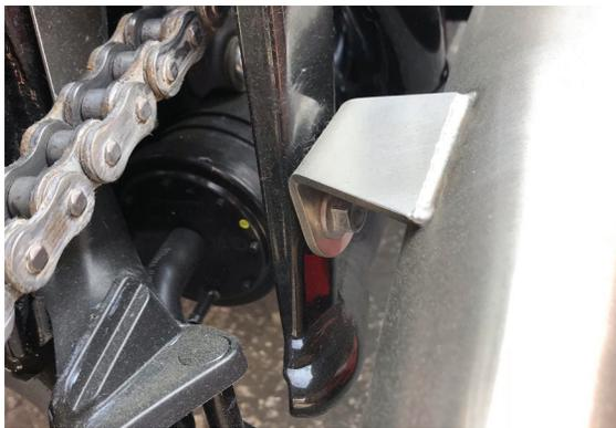
**\*Note orientation of the mounting bracket. Slotted part should be at the top.**
