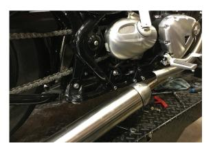
8. Use 12mm socket to remove the rear muffler mounting bracket.
