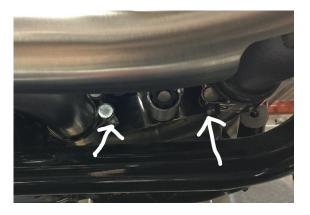
Install heat shield to tailpipe.
