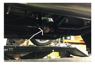
3. Place kickstand stopper bracket into position and secure with supplied 8mm allen.
