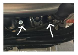
3. Use 5mm allen to remove the heat shield clamp bolt. (On the left hand side, remove the heat shield mid-section.)
