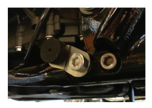
Cycle the kickstand to get the bracket into proper position, then tighten and torque to 40 Nm. (30 ft-lb)
