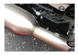
10. Go to rear mount and tighten rear mounting bolt with 12mm wrench to approx to **19 Nm (14.0 ft-lb)**
