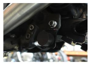
12. Before starting motorcycle, check for proper clearance between exhaust system with the frame, suspension, wiring, etc. If any problem is found, please carefully follow through the installation steps again. If problem still persists, please call **British**Customs Customer Support at (877) 999-2748.
