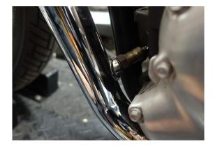
5. Use 8mm allen and remove bolt from rear of head pipes.
