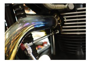
9. Separate the head pipes at the crossover pipes.
