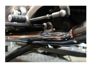
7. Use 6mm allen and loosen the crossover clamp between the head pipes, located under the engine.
