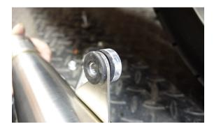
7. Install supplied clamp on the end of the muffler. Slip muffler onto the end of the tail-pipe and lightly tighten clamp.
