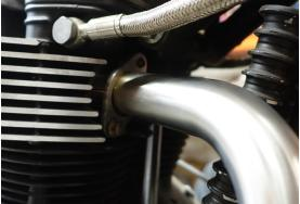
4. Align the ends of the head pipes and fit the British Customs merge pipe over them.
