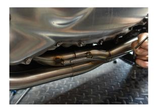
6. Install rubber grommet to muffler tab. Install aluminum insert into grommet, with insert placed on the backside of the mounting tab.
