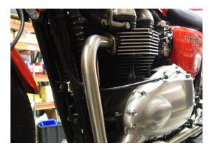
3. Place the Right-Hand header end through the area between the frame and engine, then install the collar end to the exhaust port and lightly snug flange nuts.
