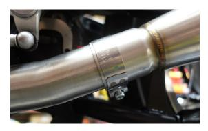
Lift muffler into position on the backside of passenger peg mount. Insert passenger peg and use 12mm socket to secure nut and torque to 19 Nm (14.0 ft-lb)
