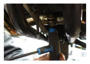
8. Use 12mm socket and remove the flange nuts at the exhaust port.
