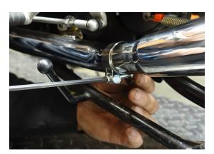
2. Use 12mm wrench to remove nut securing muffler to passenger peg.
