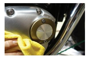
2. Using 4mm allen wrench, remove the two factory screws.
