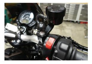
Wrap a rag around the brake reservoir and surrounding area to catch any spills. 4. Use Phillips screwdriver to remove screws securing reservoir cap. Then, carefully lift off the cap.
