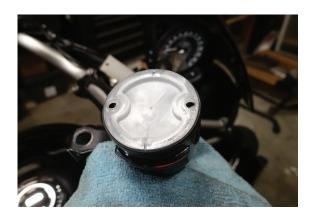
6. Use pliers to remove the spring clamp at the master cylinder.
