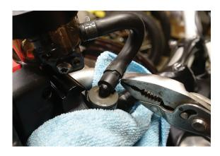
7. Remove the brake reservoir feed line from the master cylinder.
