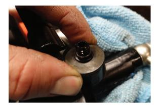
6. Screw BC brake reservoir onto the base pin.
