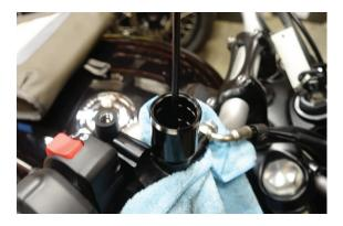
8. Use a new bottle of DOT 4 brake fluid and fill reservoir half full.
