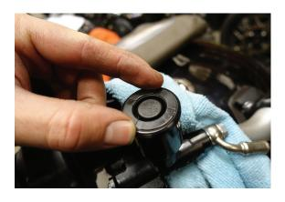
11. Install BC reservoir cap while holding the brake reservoir.
