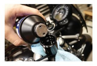
9. Set brake lever to Setting 1, where lever is furthest from handlebar. Slowly pump the brake lever to build up pressure.
