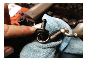
Use snap ring pliers to remove the snap ring inside the master cylinder.
