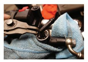
10. Remove the plastic elbow from master cylinder.
