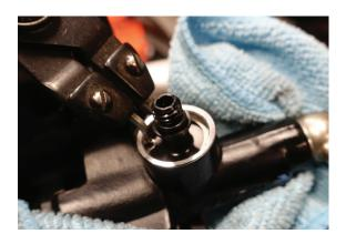
5. Install factory rubber dust cover over the base pin.
