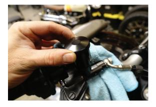
12. Pump brakes again to make sure there are no leaks.
