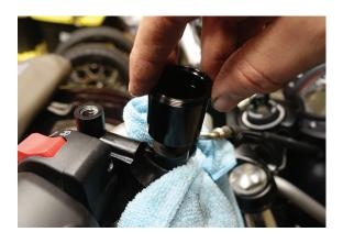
Use 4mm allen and insert into the top of the base pin. While holding the 4mm allen stationary, turn the brake reservoir clockwise until tight.
