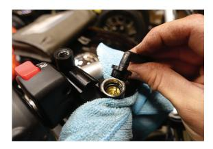
11. Use a pick and remove the o-ring in the master cylinder.
