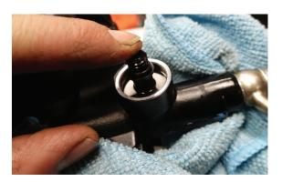
4. Use snap ring pliers and install the factory snap ring. Be sure the snap ring engages the grooves.
