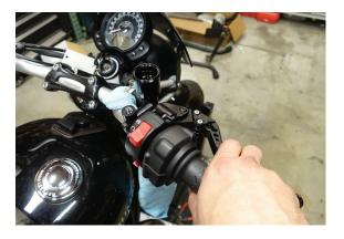
NOTE: If brake does not build pressure, bleeding the brakes may be required.
