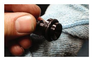
3. Press BC base pin into master cylinder until snap-ring grooves are visible.
