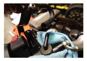
8. Remove the rubber dust cover from the master cylinder's plastic elbow.
