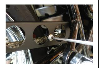
4. Use 5mm allen to install factory bolt (apply thread lock) in the rear position and snug.
