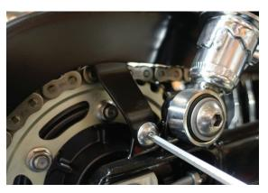
2. Use 5mm allen wrench to loosen the front bolt of the factory chain guard.
