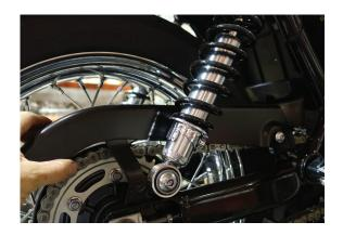
4. Remove chain guard through the rear of the bike.
