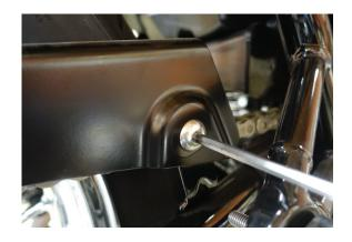
3. Support the rear of the chain guard. Remove rear bolt, then remove front bolt, and set bolts aside.
