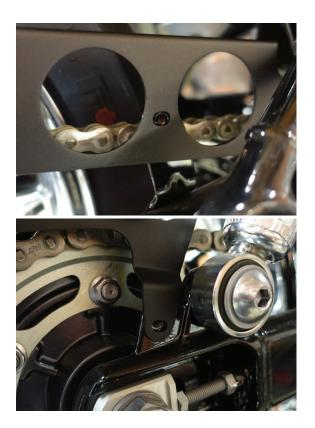
3. Use 5mm allen to install factory bolt (apply thread lock) in the front position and snug lightly.
