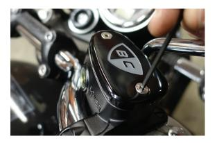
Once snug, firmly tighten each screw to 2 Nm (17 in-lbs)
