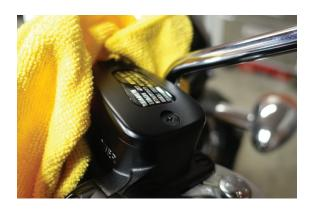
2. Loosen the two factory Phillips screws.
