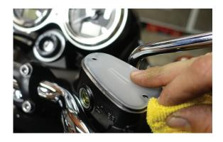
2. Install the British Customs Master Cylinder cover and insert the supplied 3mm allen screws.
