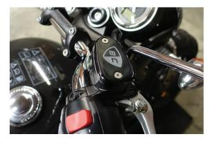
Wipe down the master cylinder and surround area with a clean microfiber cloth and rubbing alcohol to remove any fingerprints, oils, or brake fluid.
