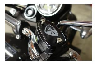
3. In an alternating pattern, tighten each screw until snug. You want even pressure on each side of the cover while tightening to prevent leaks.
