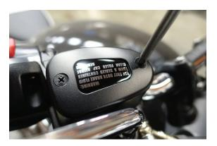
3. Carefully lift off the factory master cylinder cover. Take care to not pull out the inner plastic piece and rubber diaphragm.
