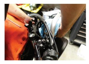
11. Pull down on the stock headlight brackets, freeing them from the underside of the upper yoke. Be sure to collect the rubber dampers if they stick to the upper yoke.
