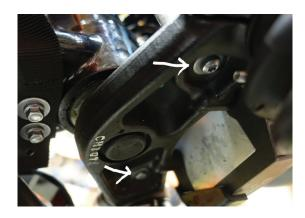
6. Use 6mm allen and loosen the upper yoke pinch bolts.
