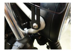
5. Use T25 Torx and remove the two screws securing the headlight bracket under the lower yoke.
