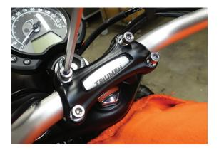
Place a clean towel over the instrument cluster, then lift and set handlebars on the instrument cluster.
