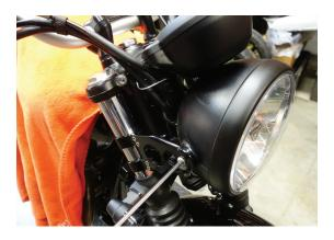
8. From the front of the vehicle, adjust the headlight and headlight ears until they are centered. Use 4mm allen and lightly tighten the 4 headlight ear screws on each side.
