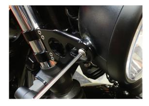
11. Use 4mm, in an alternating pattern, begin tightening the bolts 1/4 turn at a time until snug.Torque to 10 Nm (88 in-lbs.) INCH-LBS
