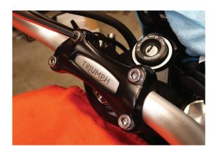
NOTE: There is an alignment cross on the front side of the handlebar. Align the cross with the handlebar riders and clamp.
