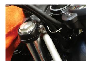
Use 6mm to remove the handlebar clamp bolts and remove the top clamp.
