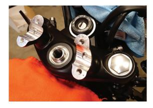
3. Use 38mm socket and tighten steering stem bolt. Torque to **90 Nm (66 ft-lbs.)**
