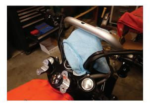
9. Use 38mm socket and breaker bar to remove the steering stem bolt.
