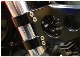
Gently place the upper yoke over the fork legs and steering stem. Press down to seat the upper yoke.
