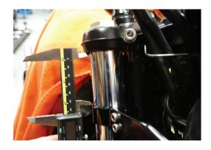
Tighten the headlight mount screws. Torque to 10 Nm (88 in-lbs.) INCH-LBS
