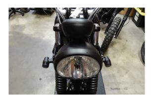
9. Check that the distance from the headlight ear to the upper yoke is the same on both sides.
