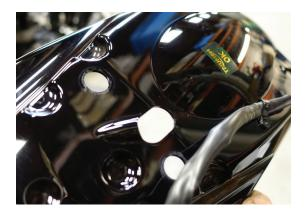
2. Use supplied spacers on back of the Pan taillight assembly. These are required for the taillight to sit properly spaced off the fender.
