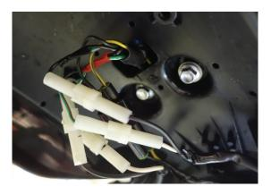
11. Disconnect the taillight harness from factory harness. Use 8mm socket to remove remaining taillight mounting bolts.
