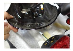
13. Pull rear light wiring from the inner fender to clear room for trimming.
