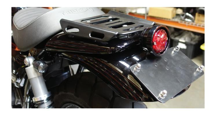
NOTE: Pan Taillight requires trimming the inner fender and removing the factory taillight and turn signals. Additional turn signals will be required for Street Use.
