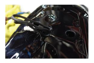
6. Install inner fender using 10mm socket, remaining nyloc nuts and washers to snug inner fender and taillight to fender. Do not tighten at this time.
