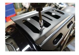
STREET SCRAMBLER: Use 6mm allen to remove the luggage rack mounting bracket and rear cowling.
