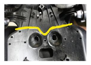
15. Use cutoff wheel to trim off back half of inner fender, removing the lights from the inner fender.
