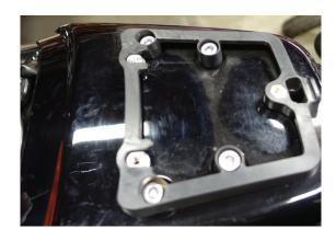
Use T30 Torx to loosen fender mounting hardware. Support rear of the fender, then continue loosening until the fender drops free.
