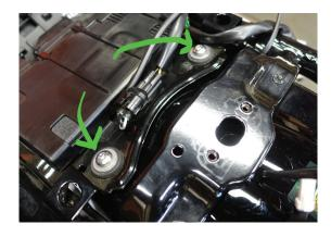
9. Use T30 Torx and snug the rear fender mounting bolts.
