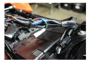
13. Tuck wiring slightly under the seat latch mount for clean install.
