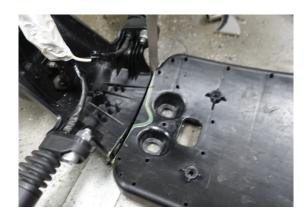
Use metal file and/or sand paper to clear off the plastic burrs and sharp edges.
