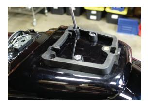
16. Use 6mm allen and tighten luggage rack mounting bracket hardware. Torque to 15 Nm (132 in-lbs) \*INCH-LBS 17. Place luggage rack on mounting bracket, use 4mm allen to secure luggage rack to mounting bracket.Torque to 8 Nm (70 in-lbs)\*INCH-LBS
