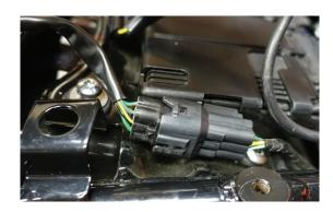
12. Connect Pan taillight harness to factory harness. Zip-tie excess wiring together.
