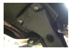
10. Disconnect wiring found under the harness cover. Use 8mm socket to remove two bolts securing the inner fender guard.
