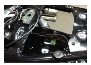
8. Use T30 Torx and snug the front fender mounting bolts.
