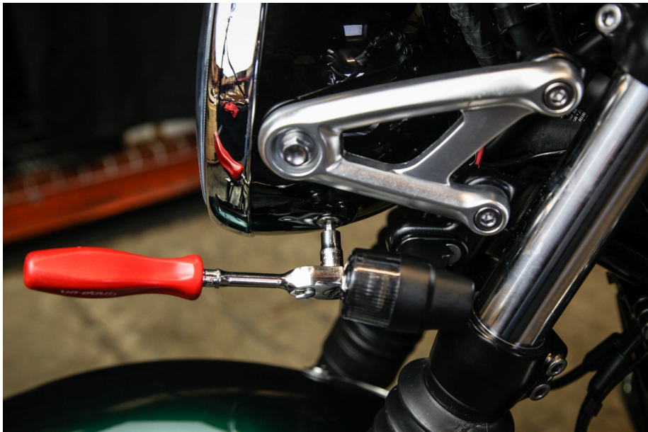
STEP 14: Use a 5mm Allen wrench to install the two screws on the bottom of the headlight bucket.
