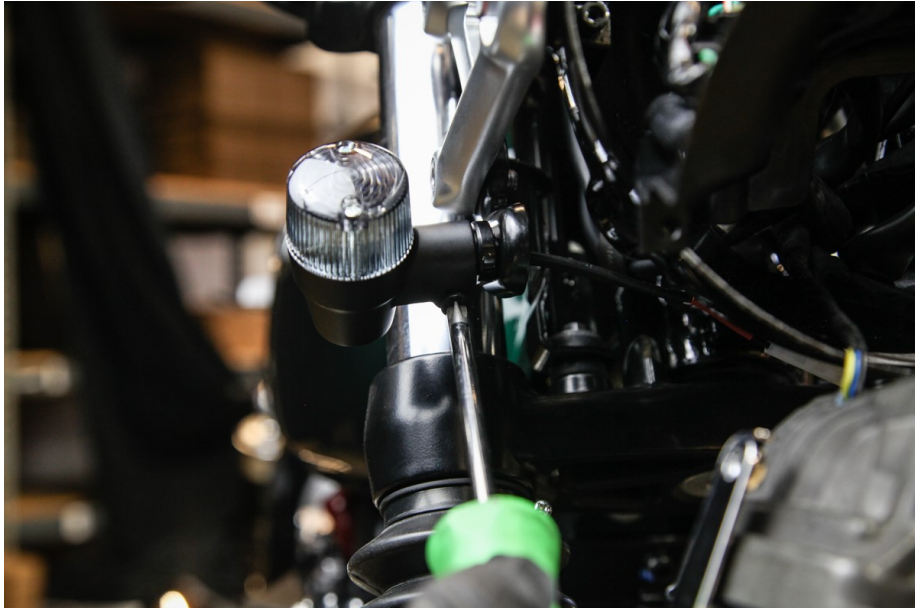
STEP 8: Mount the new Turn Signals on the turn signal bracket. Use a Phillips head screwdriver to loosen the turn signal so that it can be freely adjusted.
