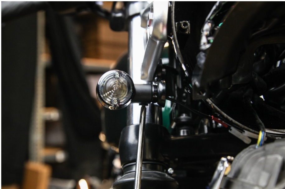
STEP 10: Adjust the new Turn Signals to the desired position and use a Phillips head screwdriver to secure them in place.
