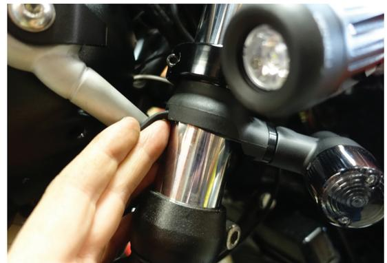
5. Slide mounting clamp down into position, making sure turn signal harness stays tucked inside the clamp.
