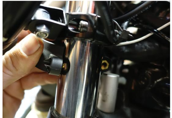
11. Use 5mm allen and remove screw securing the turn signal to clamp.
