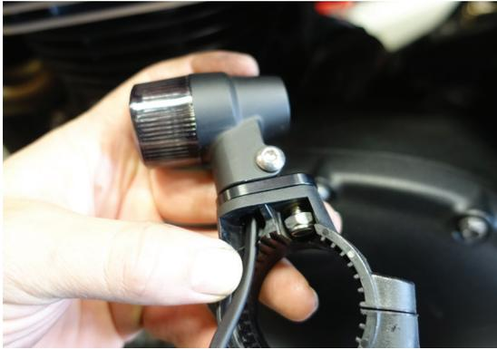
1. Feed British Customs turn signal wiring through mounting clamp. Wiring sits in the recess inside the front portion of the clamp.
