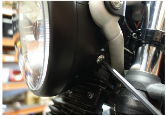
5. Pull headlight assembly from bucket. May take a little wiggle to break free. Place clean towel on top of the front fender and let headlight assembly hang.
