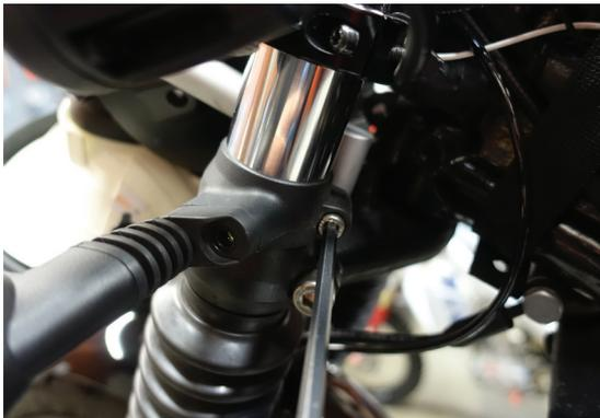
9. Slide the turn signal clamp up the fork leg to clear the headlight mount bracket.
