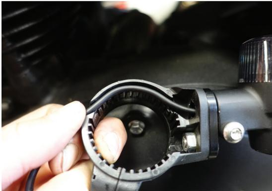
2. Use 4mm allen and secure turn signal to mounting clamp.
