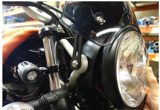
6. Use T20 Torx wrench to remove two screws holding in the inner panel.
