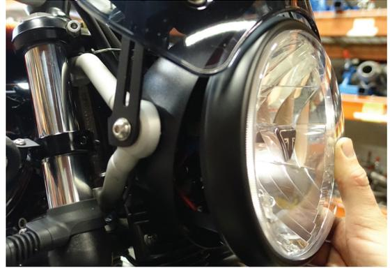
12. Use 5mm allen and secure headlight assembly in headlight housing to **4 Nm (35.4 in-lbs) INCH-POUNDS**
