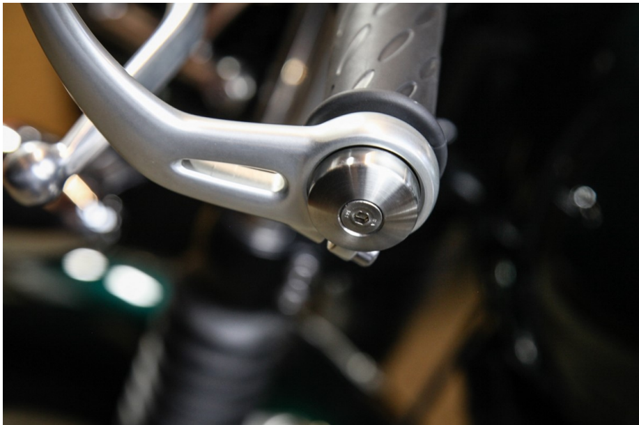
Left Stainless Weighted Bar End Installation complete!
