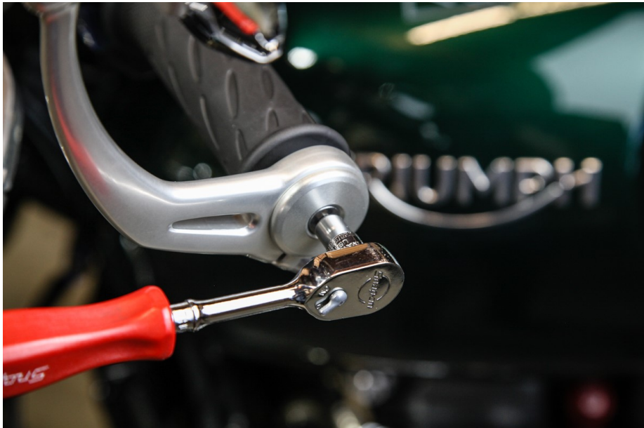
STEP 3: Use a 4mm Allen wrench to remove the left stock bar end.
