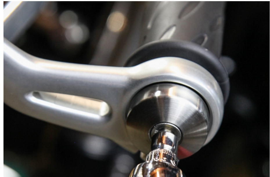
STEP 4: Clean the stock screw and apply blue Loctite to it. Use a 4mm Allen wrench to install the Stainless Weighted Bar End with the stock screw. Tighten until snug.
