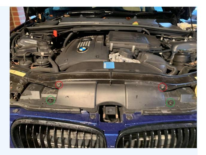
Remove Air Scoops – Unscrew 2 x T20 Screws (Red) / Undo 2 x Clips (Green)
