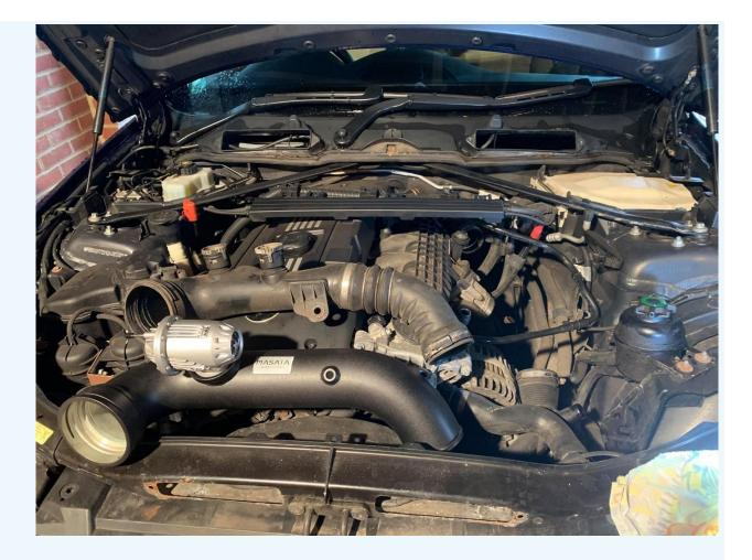
Remove OEM Chargepipe (OEM vs Masata Chargepipe with HKS Flange & HKS BOV)
