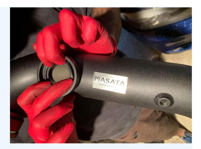
Install HKS O-Ring (You may need to stretch the O-Ring so it seats correctly into the groove)
