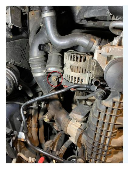
Unscrew Chargepipe Bracket (T30 Screw)
