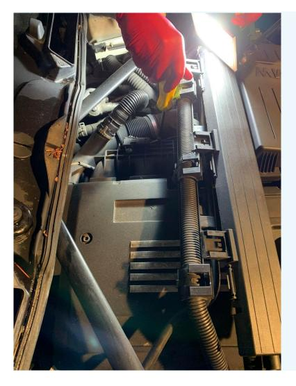
Loosen rear clamp connected to the airbox
