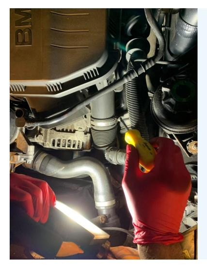
Loosen front clamps connected to the airbox
