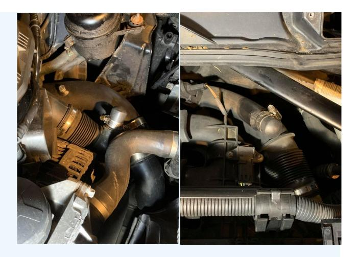
Plug Diverter Valves ports using bungs and secure with clamps x 2. Refer to photos above for the front view (left) and rear view (right)
