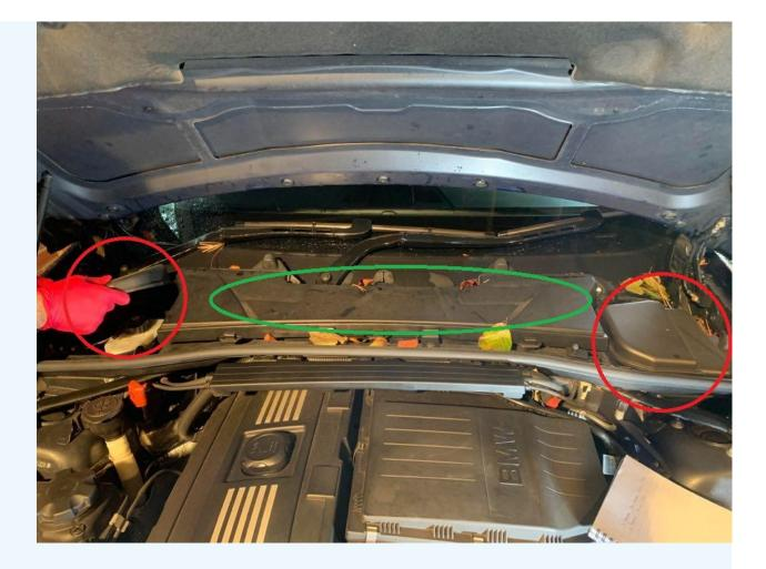
Remove Cowls(Green) and 2 x Lids (Red) - Unplug two bonnet sensor either side
