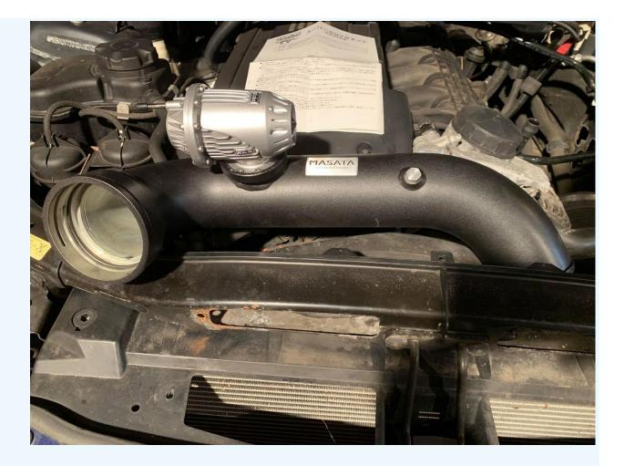
Install HKS BOV and secure it with C-Clip with a C-Clip Too. Transfer Chargepipe O-Ring from OEM Chargepipe to the Masata Chargepipe (Ensure it is seated in the Groove properly)
