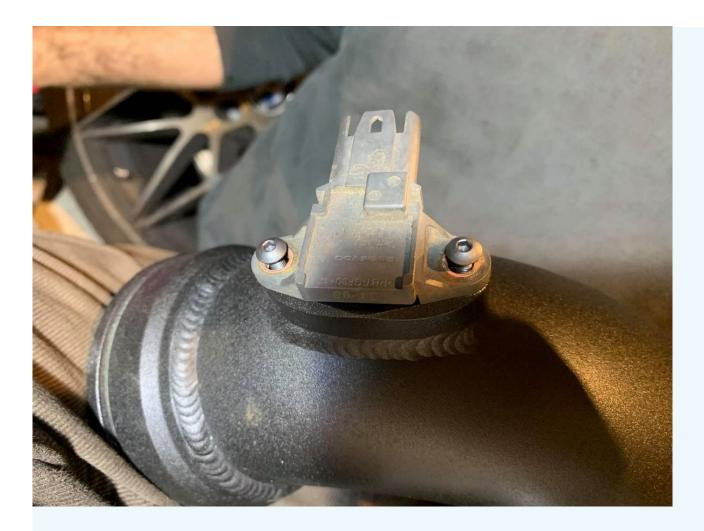
Transfer TMAP Sensor from OEM Chargepipe to the Masata Chargepipe, using the 2 x 2.5mm screws provided in the kit to secure it onto the sensor housing
