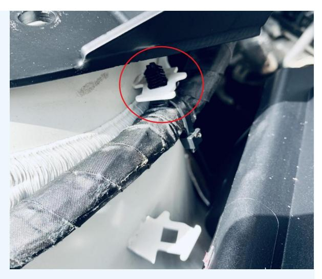
Repeat the procedure on the opposite strut tower, this will ensure that the wiring does not get trapped or interfere with the strut brace.
