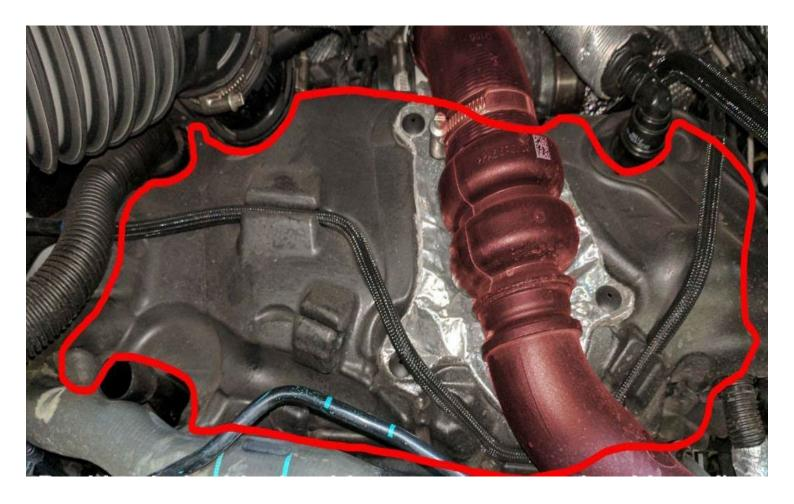
With the Boost pipe (highlighted with red glow) now removed you can now pull the rubber cover back (outlined in red) and gain access to the fuel rail
