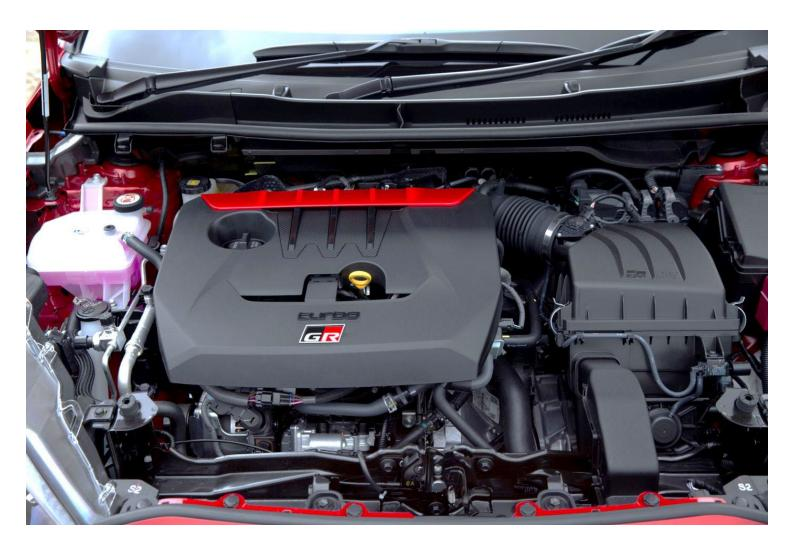
• Remove the plastic engine cover. This usually pulls off with a firm tug. On certain models the cover is secured with bolts. If this is the case, remove the bolts and lift off the engine cover.
