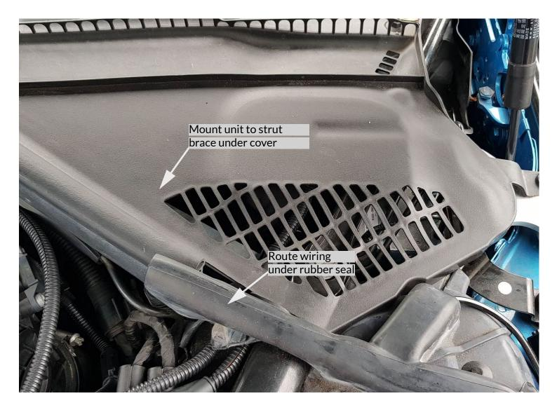
• The unit mounts very nicely in the scuttle tray underneath the plastic cover as pictured above. It can be secured to the metal strut brace underneath.
