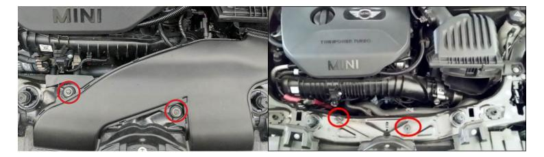
• Remove the two bolts holding in the intake duct in order to gain access to the boost sensor (highlighted in red)
