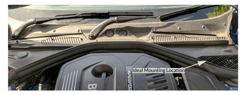
The unit is best mounted under the plastic cover on the right hand side of the bay as you look at it (left side of the vehicle). There is a black metal brace under here ideal for securely strapping the unit to.
