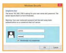
Connect to uSwitch by entering the factory default IP address (http://192.168.1.199) into the address bar on your computer's browser.
