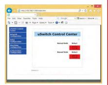
Verify relays are working by pressing buttons 1 and 2 on the web relay control page.
