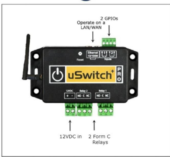
Connect a 12VDC 1 Amp power supply to the + and - Terminals on uSwitch. (regulated power supply recommended). The power supply should be rated to meet the operating current of the uSwitch Pro+
