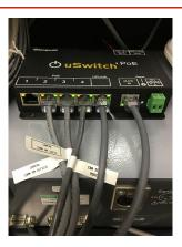
The uSwitch PoE with Watchdog capabilities pings your local LAN devices such as IP cameras as well as url's and IP addresses on the WAN. If they are unresponsive, it then automatically reboots your network devices with no human intervention. The uSwitch POE is also accessible using any web browser. When logging in, you can reboot the POE ports manually or control the onboard relay from anywhere.
