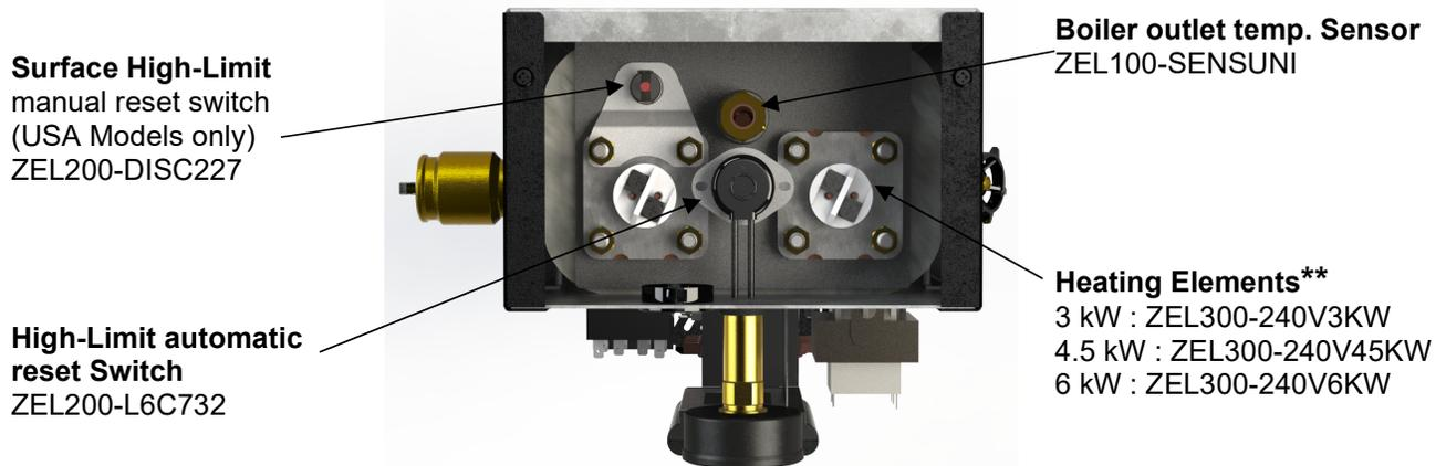
Figure 18 : Replacement Parts (Top view)
