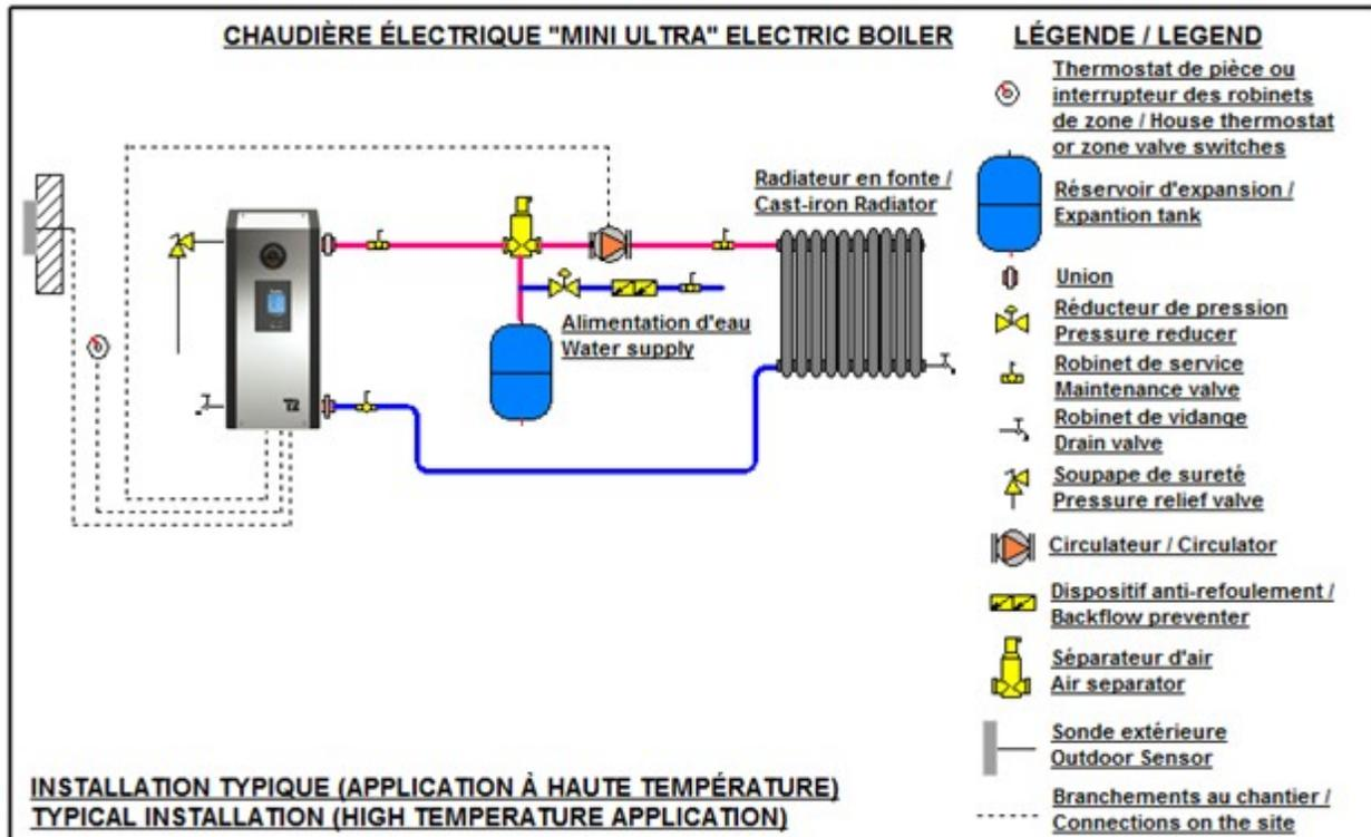
Figure 5 : Typical installation on high temperature application
