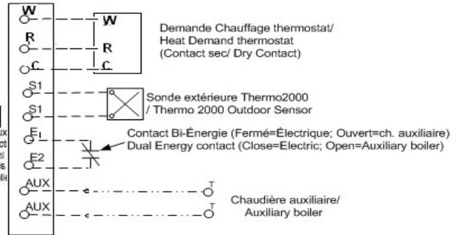
Figure 10 Connexions without three way valve
