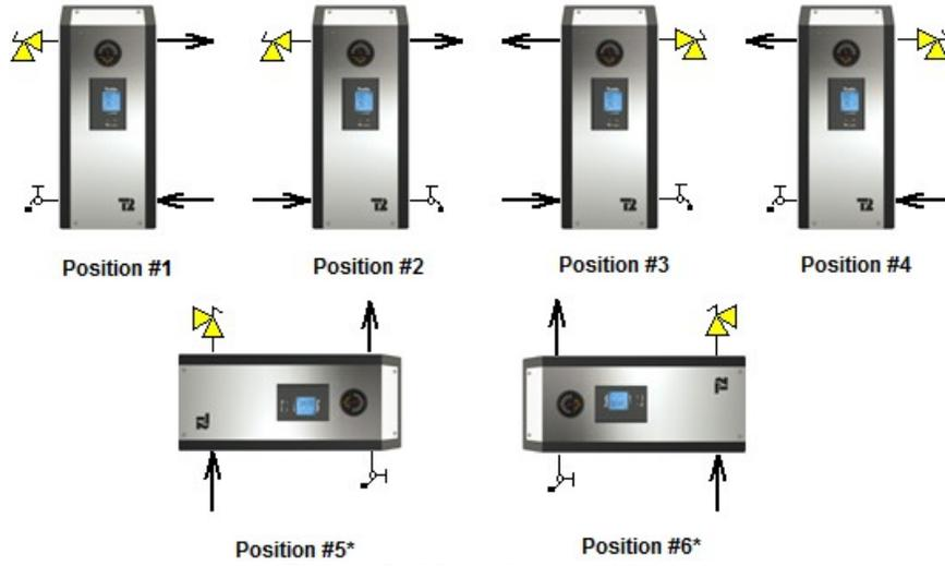
**Figure 2 : Mounting positions**
