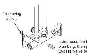
.depressurize the plumbing, then push Bypass Valve body toward softener
