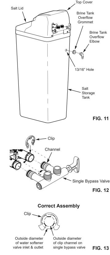
**NOTE:** Be sure all 3 tabs of the clip go through the matching holes on the water softener valve inlet or outlet, and fully into the channel on the single bypass valve. Make sure that the tabs are fully seated.
