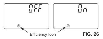
**SALT EFFICIENCY:** When this feature is ON, the water softener will operate at salt efficiencies of 4000 grains of hardness per pound of salt or higher. The softener may recharge more often using smaller salt dosage and less water. This softener is shipped with the efficiency feature set OFF. Use the  $\triangle$  UP or  $\nabla$  DOWN buttons to change between OFF and ON. An efficiency icon will be displayed when this feature is ON.
