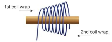
When wrapping on copper pipe, make sure the coils are always wrapped **around the pipe** in the same direction.
